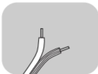
**IMPORTANT:** Typically, one side of the wire is smooth. Connect this side to the - (black) connection. The other side has a rib or stripe or other marking. Connect this to the + (red) connection.
